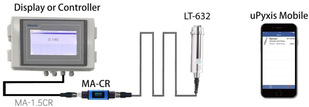
Figure 5 - LT-632 and MA-CR Bluetooth Adapter Powered By Connected Display, Controller or PLC
