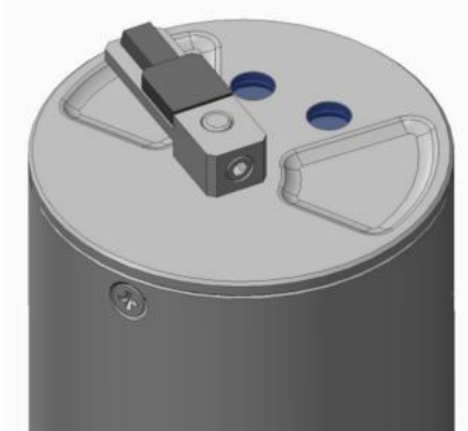
Figure 29 Set wiper arm to horizontal position
