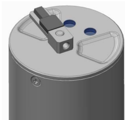
Figure 32 Install the new wiper arm
