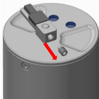
Figure 30 Remove the M2 screw
