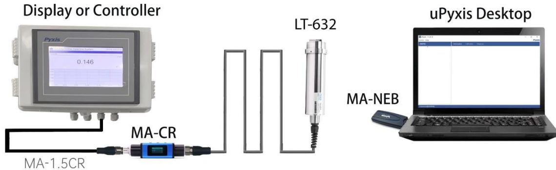
Figure 17 - Connect the LT-632 to a computer via Pyxis MA-CR and MA-NEB adapter
